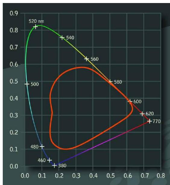
Figure 1: Surface Colors within the 1931 CIE Chromaticity Diagram
