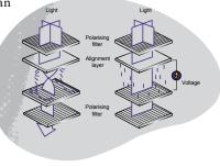
If an electrical voltage is applied, however, the liquid crystal molecules align themselves parallel to the electric field. The 90° helix is reversed and the liquid crystal molecules are parallel to the incoming light and let it pass through the layer without altering the direction of polarisation. The non-rotated beam of light meets the second, rotated polarising filter and cannot pass through. As a consequence the corresponding pixel remains dark.
