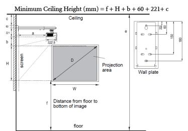
• The dimensions are based on the BenQ wall mount (P/N: 5J.J4V10.001).
